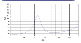
Note: Electrical impedance measured coupled to TD-365 horn
