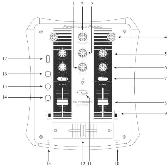
**1. CUE LEVEL VOLUME CONTROL -** This knob adjusts the headphone volume output level. Turning the knob in clockwise direction will increase headphone volume output.
