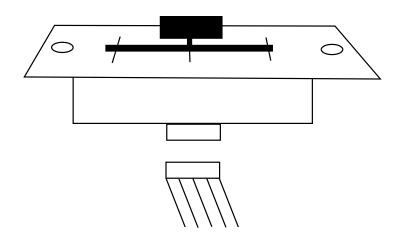
The crossfader is "Hot Changeable" which means it may be replaced at any time, even when power is applied. Only replace with American Audio Feather Fader Plus. Replacing with any other model fader may seriously damage your mixer.
