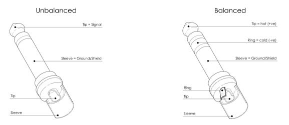
For these applications the unit provides 1/4" TRS and XLR connectors to easily interface with most professional audio devices. Follow the configuration examples below for your particular connection.
