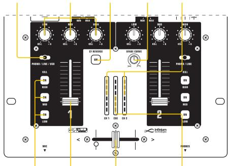
KILL buttons remove high, mid and low frequencies from A or B crossfader mix CHANNEL FADER controls volume of channel in overall mix CROSSFADER fades between sources assigned to either side MASTER
