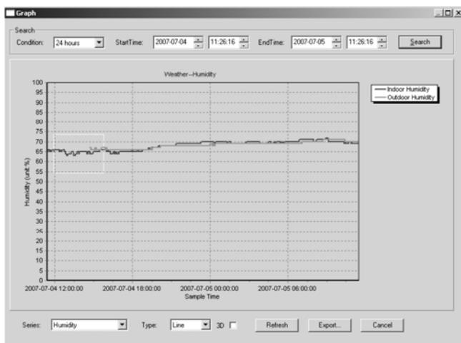
This window gives you a plotted graph. Zoom into the graph by selecting the desired area with your mouse. Select the [3D] option to display the graph in 3D format.
