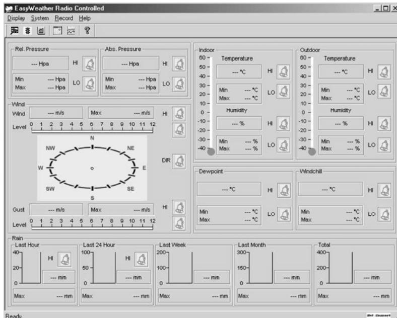
All settings from the receiver are mirrored into the software. Once you have set the receiver, there is no need to make any setting changes on the PC. However, modifications can easily be made through the EasyWeather software if needed. Those modifications will automatically be saved into the receiver.
