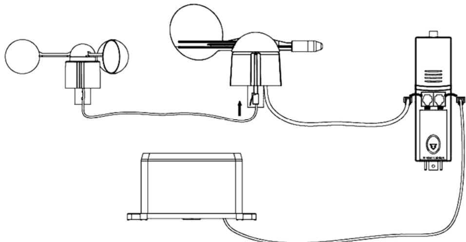
Install your outdoor weather station on a suitable location minding the wind direction markings. Connect the anemometer to the wind vane phone jacket. Connect the wind vane to the thermo-hygrometer WIND phone jacket. Connect the rain sensor to the thermo-hygrometer RAIN phone jacket. Finally, insert 3 x AA batteries into the weather station respecting the polarity.
