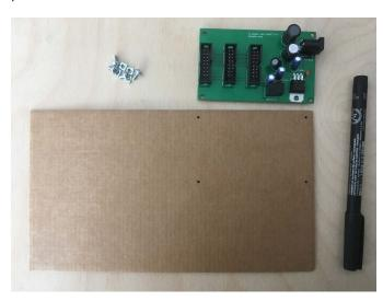
With the help of a screwdriver open these 4 holes, place the board on top and add the bolts.
