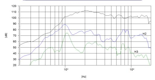
Note: On axis frequency response measured with CD-10/Fe standing on infinite baffle in anechoic chamber, 1W @ 1m
