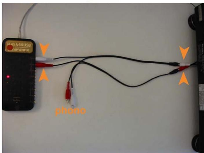
Connect the Y to each rca of your turntable cable. For each Y, connect a cable to the input of your audio card and a cable to phono input of your audio mixer.
