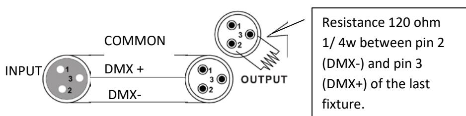
Termination reduces signal errors. To avoid signal transmission problems and interference, it is always advisable to connect a DMX signal terminator.
