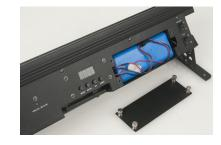
3. Carefully pull out the battery connector cables.
