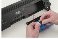
5. Carefully disconnect the battery cables.
