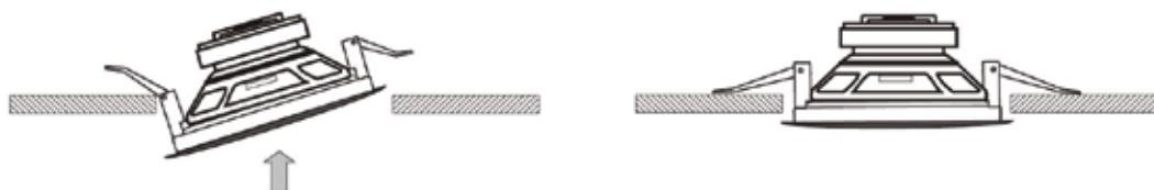
Step 1: Measure and mark the hole that you will drill into the ceiling. Please respect strictly the indicated dimensions of the mounting hole. If the hole is too big, the speaker might vibrate.
