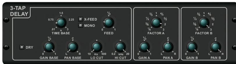
The **3-TAP DELAY** in the X32 records the input signal and then echoes it back after a user-definable period of time and number of repeats. What makes the stereo and triple delay useful and outstanding is the linked tap-timing and musical choice of echo patterns. Use the 3-TAP DELAY to fatten up vocals and instruments, or to add an enhanced spatial element to any performance.
