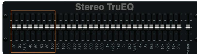
Unlike typical graphic EQs, our **STEREO TruEQ** delivers the exact frequency response for the new fader setting, taking neighboring fader settings into account – for surgical and responsive filtering or general room equalization (Modeled after BEHRINGER UltraCurve DEQ2496). The XR12 can provide up to 16 mono graphic EQs – one in each of the 6 Aux Buses and Main LR, plus 8 additional mono GEQ effects (4 stereo) that may be inserted into channels.
