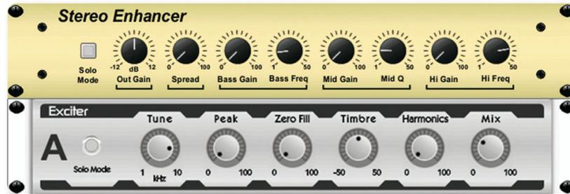
**ENHANCERS** let you emphasize the Bass, Midrange and Hi output at selectable frequencies, allowing you to generate maximum punch, clarity and detail – without turning up the overall volume. (Inspired by SPL Vitalizer\*)
