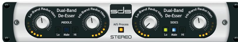
The **DE-ESSER** is a “must-have” tool for reducing the amount of sibilance in vocal mics while adeptly preserving the natural voice timbre of a performance. Use it to enhance the smoothness of the upper mid to high frequencies in vocals as well as drum overheads and strings, etc. (Inspired by SPL 1219\*)
