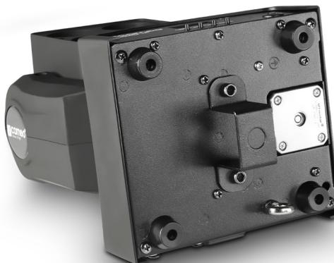
**EN** Thanks to the integrated rubber feet, the spotlight can be placed in a suitable location on the stage floor etc. Mounting on a truss is performed with the help of the supplied omega mounting bracket; secure the device with a suitable safety rope to the safety screw eye. Fix both firmly onto the base plate of the spotlight, suitable screws are included in the delivery. NOTE: Overhead installation should only be carried out by trained personnel.
