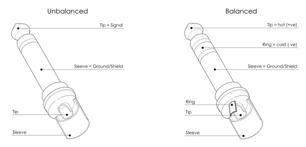
For these applications the unit provides 1/4" TRS and XLR connectors to easily interface with most professional audio devices. Follow the configuration examples below for your particular connection.
