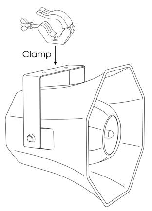
The MHS-80S can be mounted to any kind of truss with a clamp.
