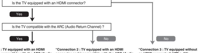
"Connection 1 : TV equipped with an HDMI connector and compatible with the ARC (Audio Return Channel)" ((F) p. 51)
