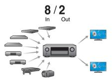
This unit is equipped with 8 HDMI inputs and 2 HDMI outputs enabling connection to various HDMI compatible devices such as Blu-ray Disc players, game consoles and HD video camcorders. This unit is equipped with 2 monitor outputs, enabling you to project the same image at the same time using this unit.
