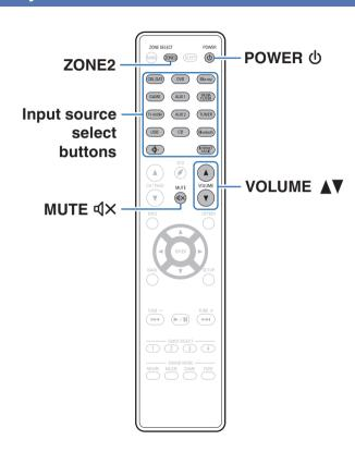
1 Press ZONE2 to set the operating zone to ZONE2 with the remote control.
