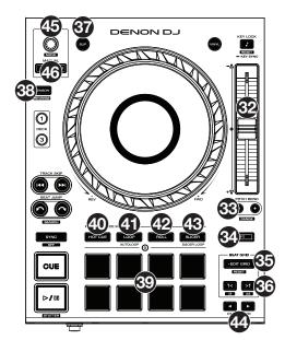
36. **Grid Marker:** When beat grid editing is enabled, press either of these buttons to move a downbeat marker backward or forward based on the current analyzed grid.
