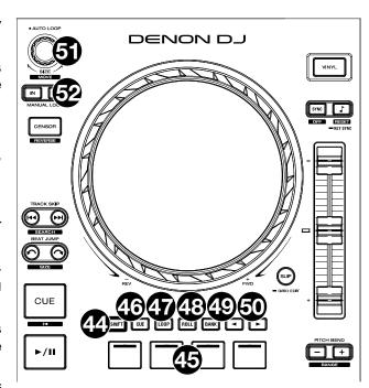
Press this knob to activate or deactivate an automatic loop at the current location of the track.
