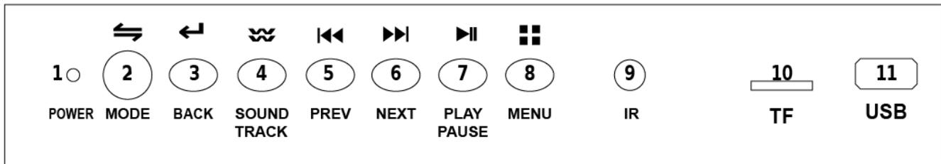
1. POWER Led: lights up when the MP5 player is switched on via the MP5 POWER switch (20) on the rear panel
