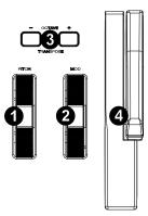
4. **Keybed:** The velocity-sensitive keyboard is not only the primary method of sending Note On/Off and velocity data when performing. It is also used to access extended programing functions listed along its upper edge.
