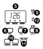
TEMPO: Tap this button to set Oxygen 25's tempo. Press and hold this button and use the < and > buttons to make incremental changes to the tempo.
