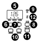
TEMPO: Tap this button to set Oxygen 61's tempo. Press and hold this button and use the < and > buttons to make incremental changes to the tempo.
