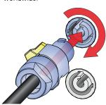
**CAUTION**: The AC Input connector should not be engaged or disengaged when under load or live.
