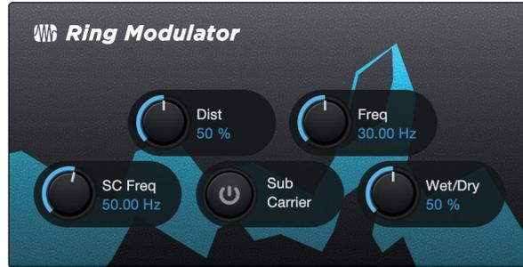
1. **Dist.** Controls the amount of distortion from zero to over-the-top.
