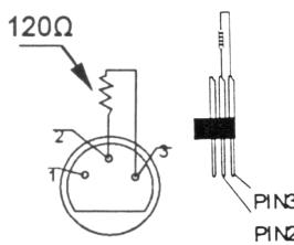
A DMX terminator is recommended for installations where the DMX cable has to run a long distance or is in an electrically noisy environment (e.g. discos). The terminator prevents corruption of the digital control signal by electrical noise. The DMX terminator is simply an XLR plug with a  $120\Omega$  resistor between pins 2 and 3, which is then plugged into the XLR output socket of the last device in the chain.
