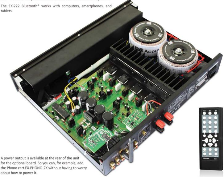
The EX-222 is dual power supply equipped, using two 200 VA Toroidal transformers. The amplifier stages share the same structure with famous EX-302, but with a doubled capacitive decoupling and a higher voltage level for final stages.
