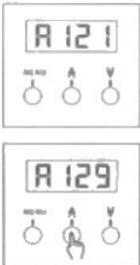
1. The segment display shows the last DMX address used. If you've select address 1, then the display segment will show 1.
