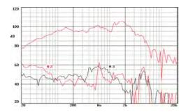
Note: on axis frequency response measured with loudspeaker standing on infinite baffle in anechoic chamber,  $1w \otimes 1m$ .
