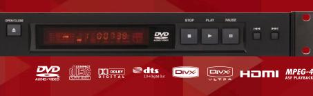
The DV-D01U is a HDCP-compliant 1-U rackmountable single disc player with a powered loading tray. It reads DVD Video, DVD Audio (2-channel only), Video CD, CD-DA, MP3, WMA, WAV, JPEG, ASF, MPEG-2/MPEG-1 and DivX. Properly finalized DVD+R/+RW media (video format discs only) can also be played back.
