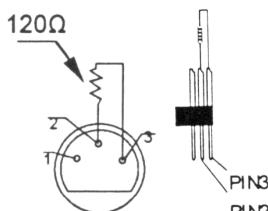
A DMX terminator is recommended for installations where the DMX cable has to run a long distance or is in an electrically noisy environment (e.g. discos). The terminator prevents corruption of the digital control signal by electrical noise. The DMX terminator is simply an XLR plug with a 120Ω resistor between pins 2 and 3, which is then plugged into the XLR output socket of the last device in the chain.
